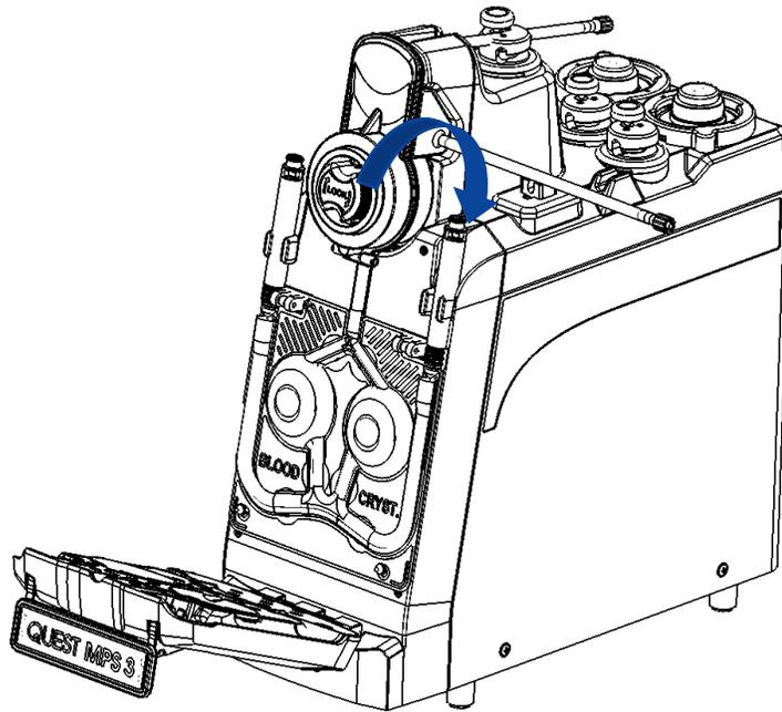
Figure 82: MPS 3 Locking Knob Engagement
