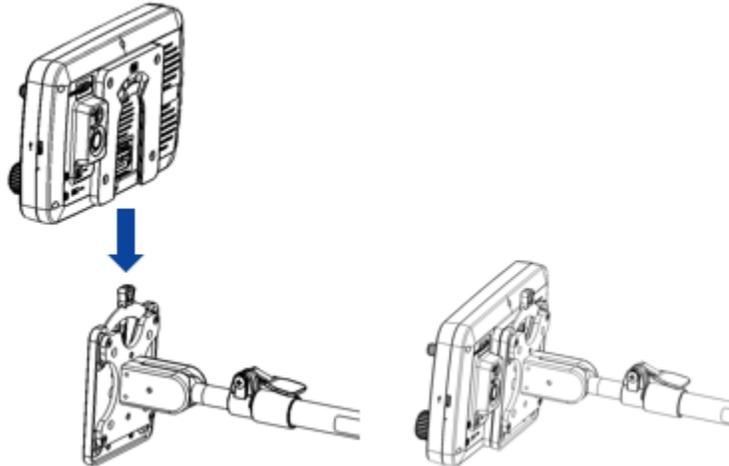
*Figure 22: Connect Controller to Arm using Quick Release Adapter*
