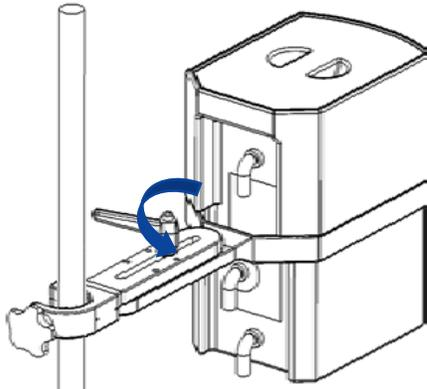
*Figure 16: Set Position of Reservoir Bracket*
