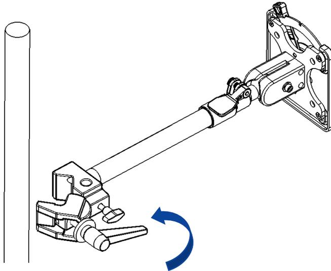
Figure 20: Loosen Pole Clamp and Position Clamp over Pole
