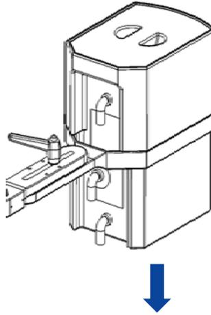
*Figure 15: Insert Reservoir into Bracket*
