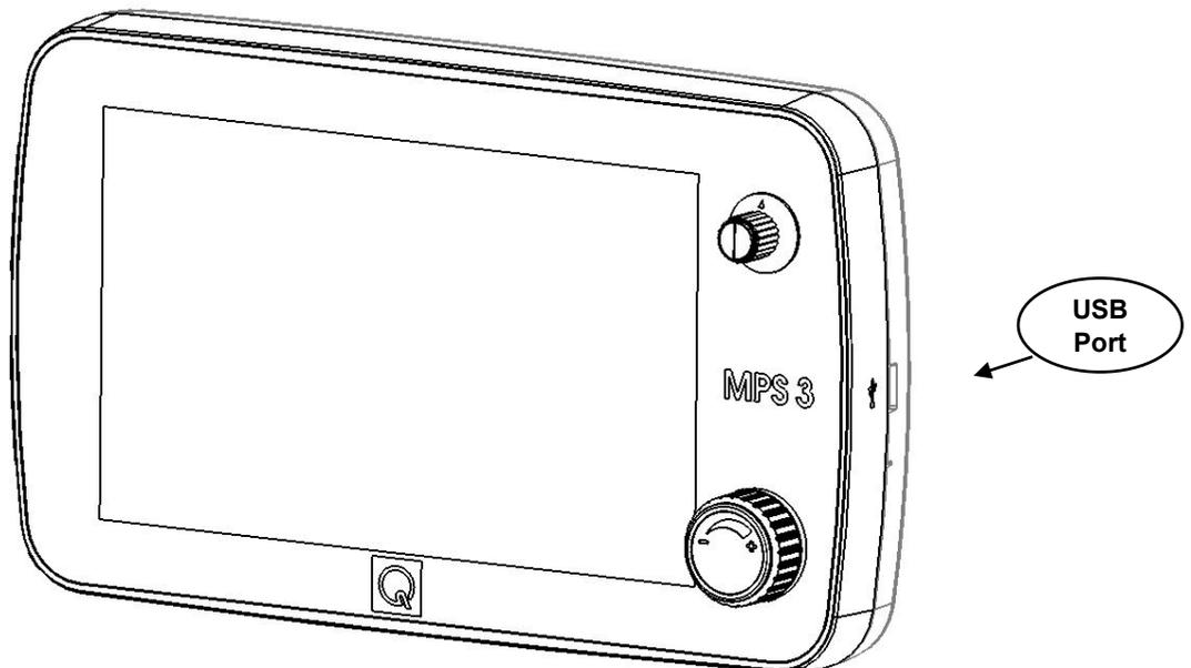
Figure 154: USB Port in the Controller
