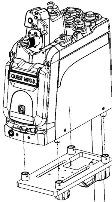
Figure 11: Install Console to Pole Mount Adapter
