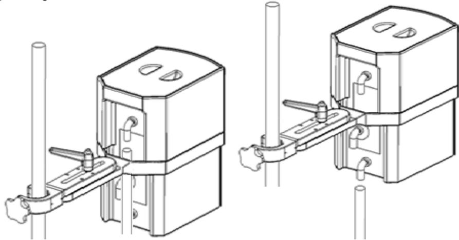
Figure 17: Install Tubing to Reservoir
