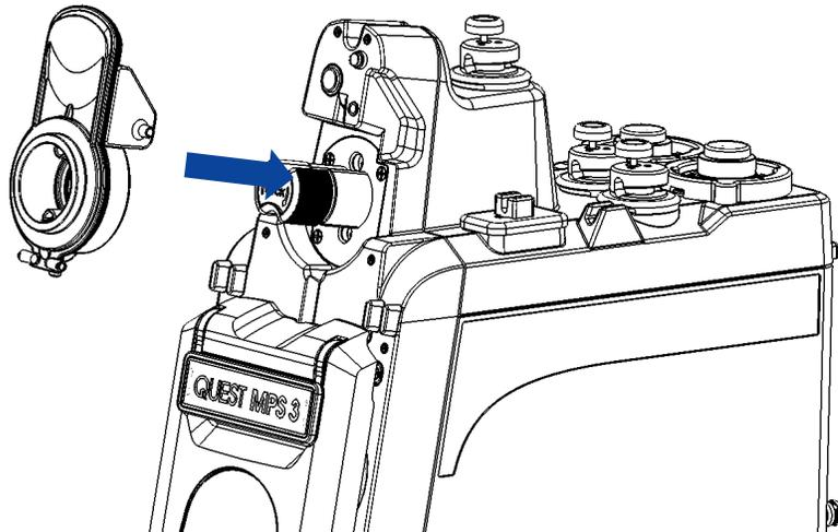
Figure 159: Console and Hypothermic Reservoir Drain Ports
