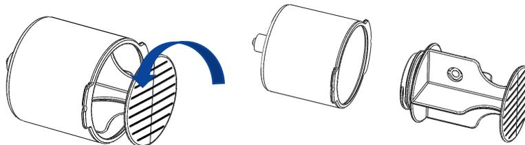
Figure 95: Plunger Removal
