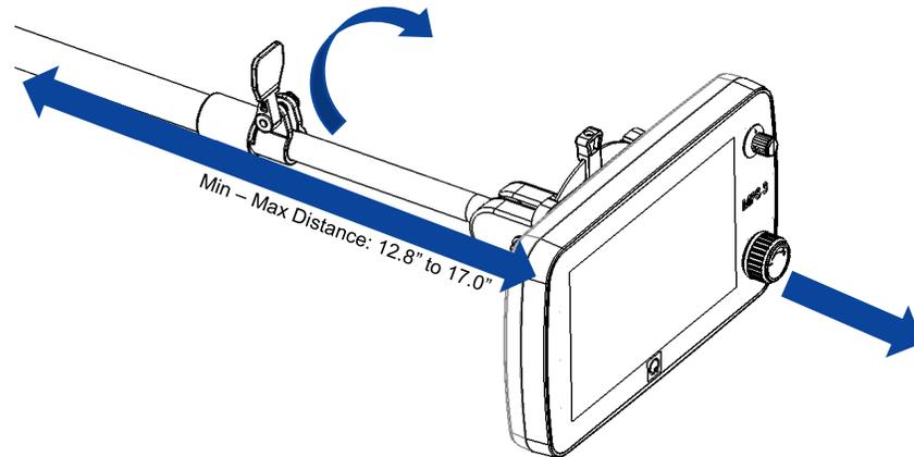
Figure 23: Loosen Telescoping Clamp to Extend Arm
