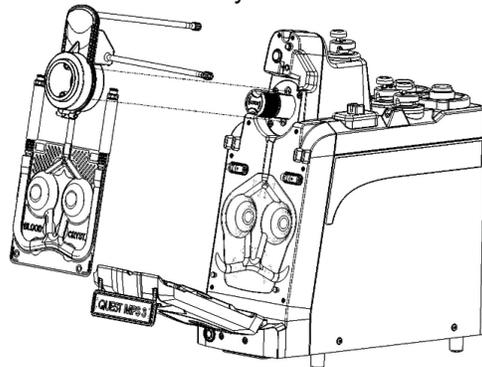
Figure 104: Delivery Set Removed from the MPS 3 Console
