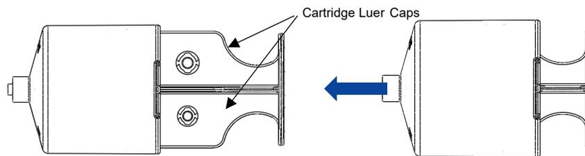
Figure 94: Fully Insert Plunger in Cartridge
