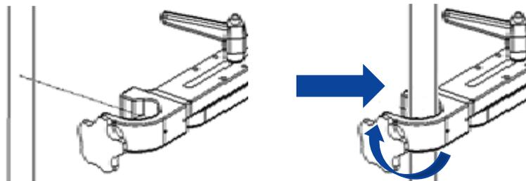
Figure 14: Secure Reservoir Bracket to Pole
