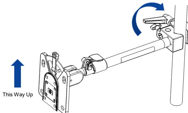
Figure 21: Tighten Pole Clamp to Secure Mounting Arm
