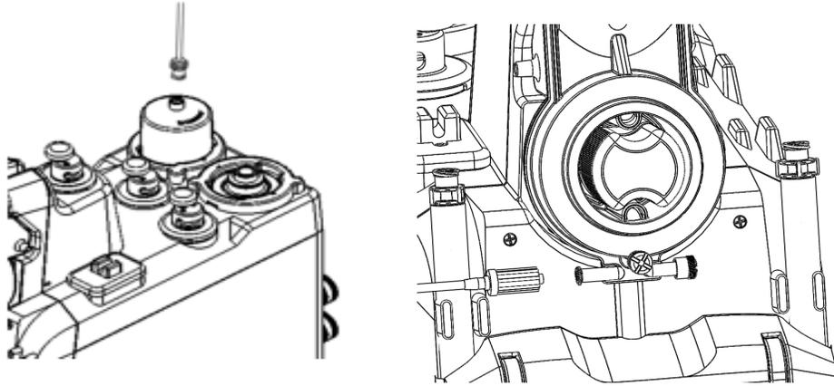
Figure 98: Connect check valve to heat exchanger
