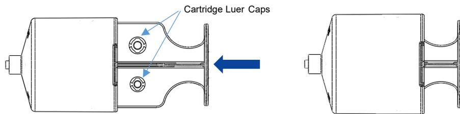
Figure 87: Fully Insert Plunger in Cartridge
