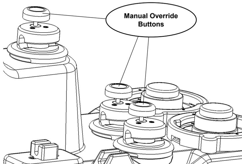
Figure 157: Delivery and Vent Valve Manual Override
