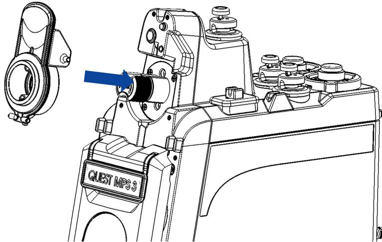
Figure 32: Console and Hypothermic Reservoir Drain Ports
