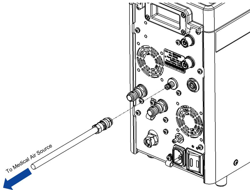
Figure 33: Install Medical Air Fitting
