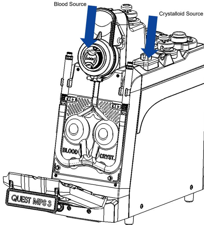
Figure 85: MPS 3 B / C Cassette Source Lines
