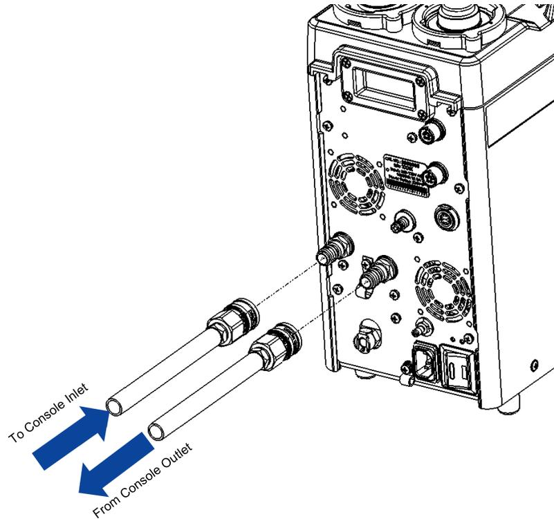
Figure 29: Connect Reservoir Tubing to Console
