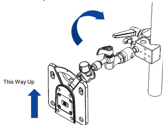
Figure 25: Tighten Pole Clamp to Secure Mounting Arm
