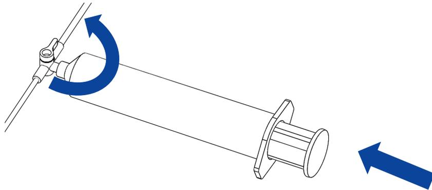
Figure 93: Cartridge filling
