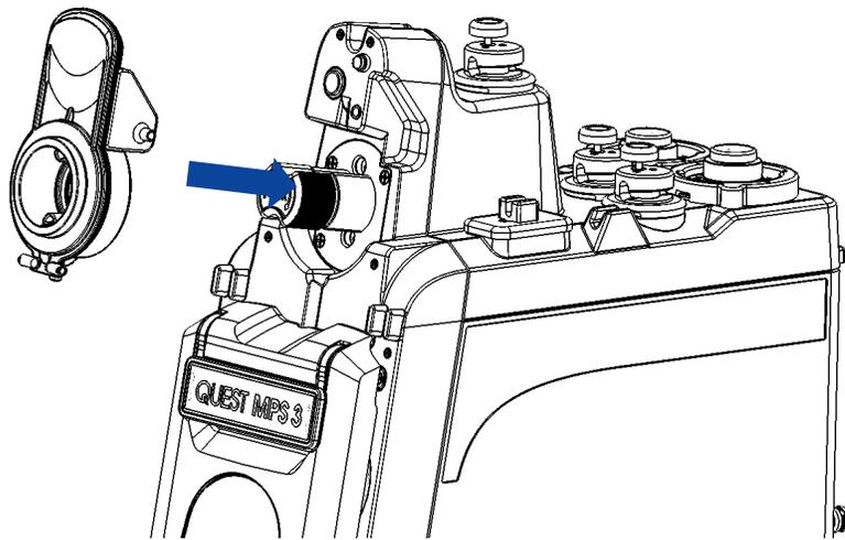
Figure 30: Installing Water Circuit Adapter
