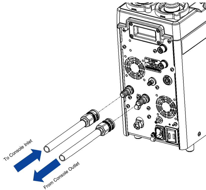
Figure 19: Connect Reservoir Tubing to Console
