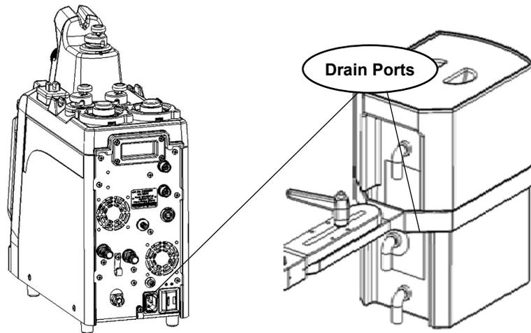
Figure 158: Console and Hypothermic Reservoir Drain Ports
