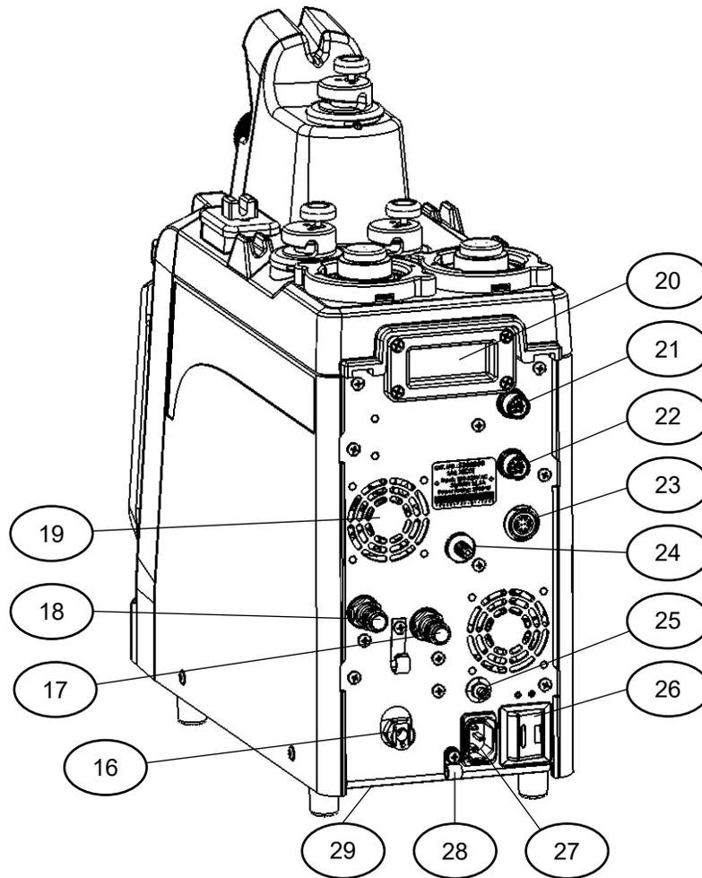
Figure 2: MPS 3 Console Rear Panel
