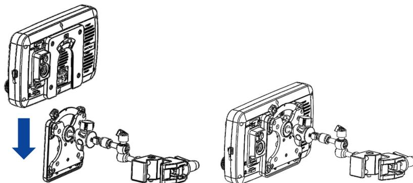
Figure 26: Connect Controller to Arm using Quick Release Adapter
