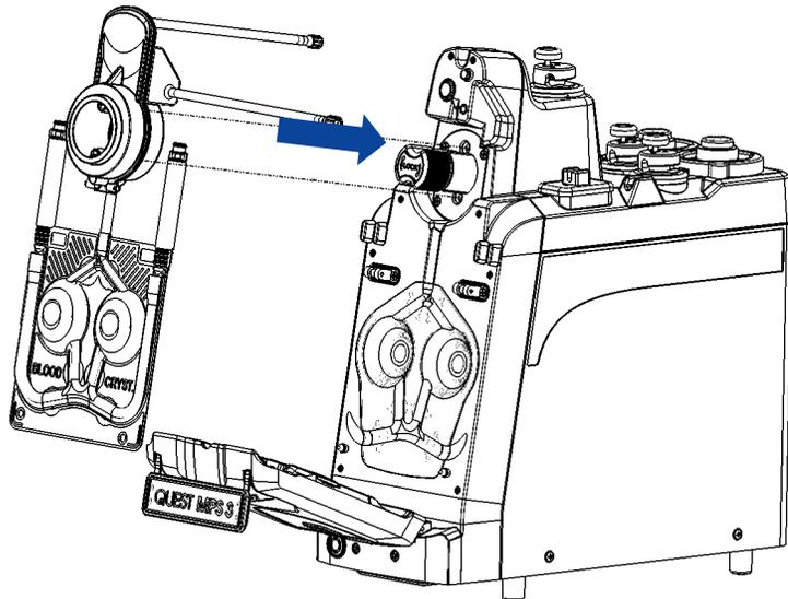
Figure 81: MPS 3 Heat Exchanger Installation
