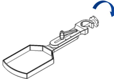
Figure 13: Loosen Pole Clamp on Reservoir Bracket
