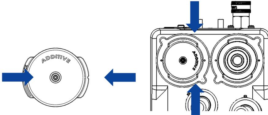
Figure 96: Align the Additive Cartridge
