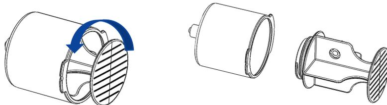
Figure 88: Plunger Removal
