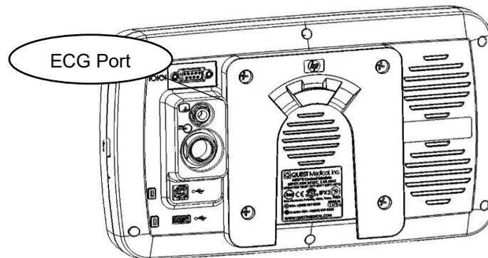
Figure 35: ECG Port on MPS 3 Controller
