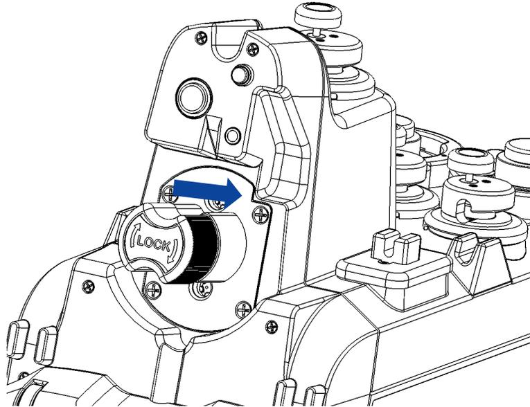
Figure 31: Manual Purge of Circulation System
