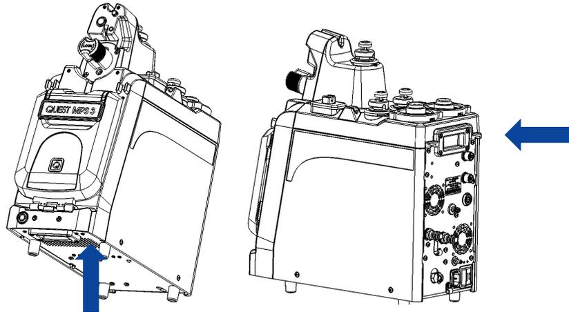
Figure 6: Lift Console with Handles
