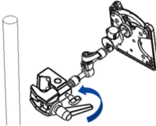
*Figure 24: Loosen Pole Clamp and Position Clamp over Pole*
