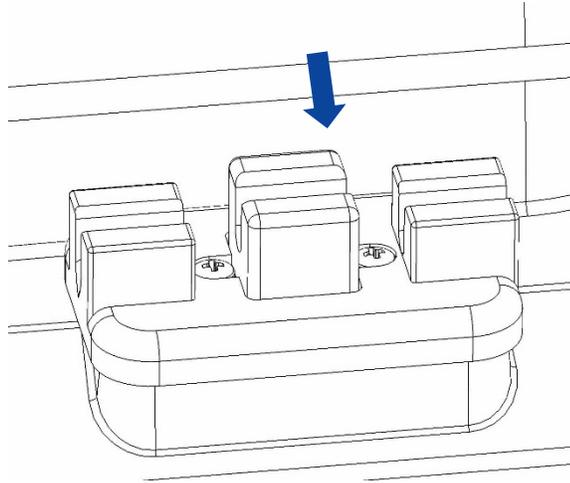
Figure 86: MPS 3 Air in Line Sensor Engagement
