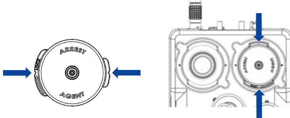
Figure 89: Align the Cartridge
