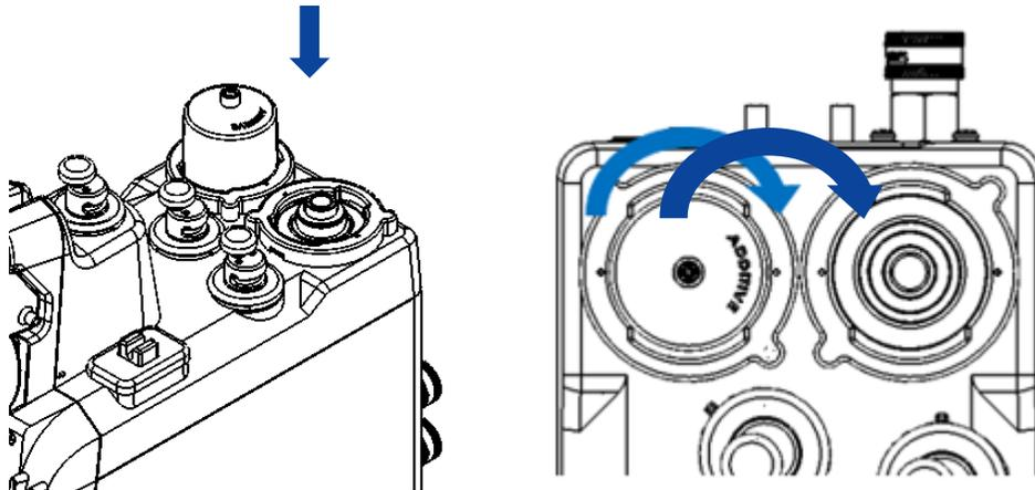
Figure 97: Secure Additive Cartridge to Console
