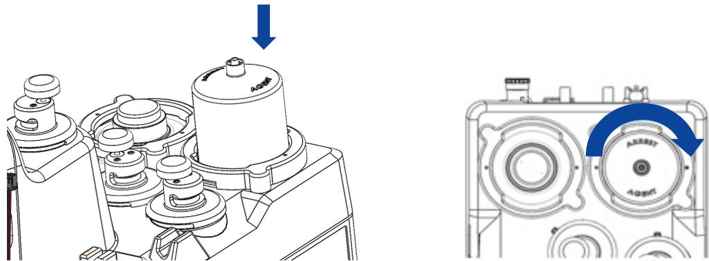
Figure 90: Secure Cartridge to Console
