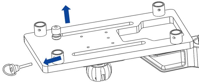
Figure 8: Remove Locking Foot from Pole Mount Adapter
