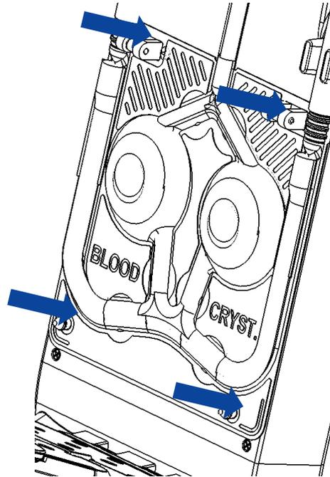
Figure 84: MPS 3 B / C Cassette Loading
