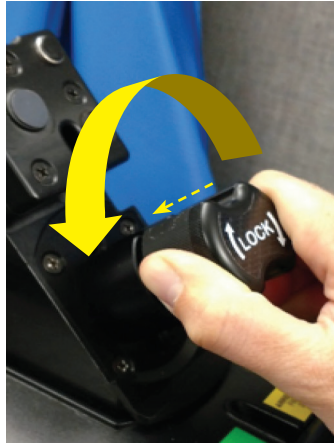
1. Push down on the knob and rotate it counter-clockwise 360 degrees until it stops rotating. (Locking knob will extend outward)
