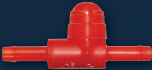
VRV-II [REF] 4003103 | 4003203 (Non-Sterile) Relief pressure: (-) -150 mmHg | (+) 340 mmHg (Avg.)
